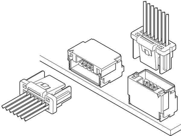
**1.0mm pitch secure lock type connector. This low insertion force type connector realizes easier mating operation. The basic concept of the contact part of this connector is equivalent to the performance proven SHL connector.**
