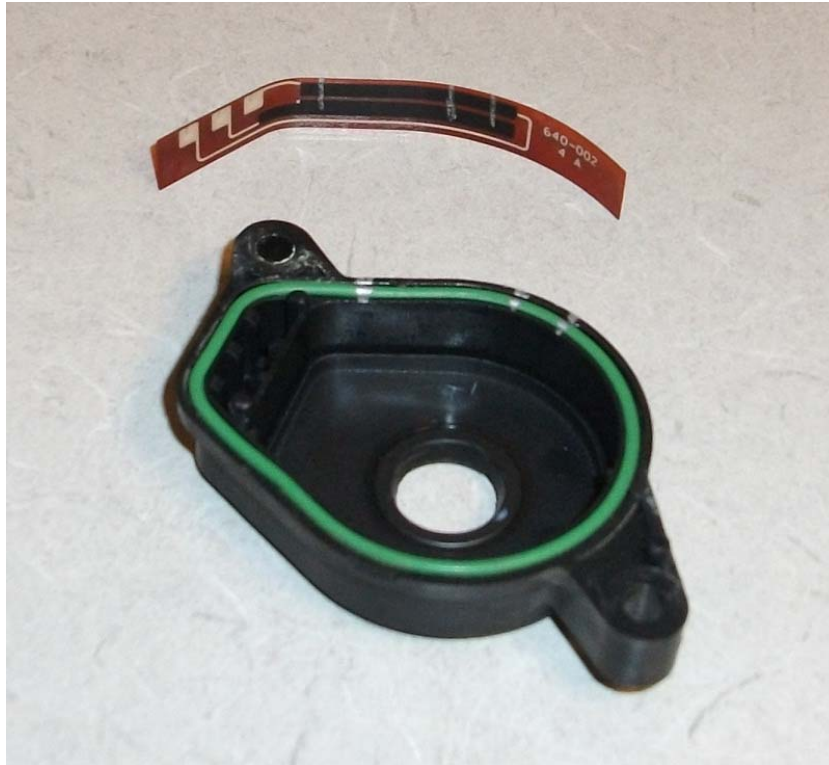
Figure 5: Resistive strip fits into the sensor housing.
