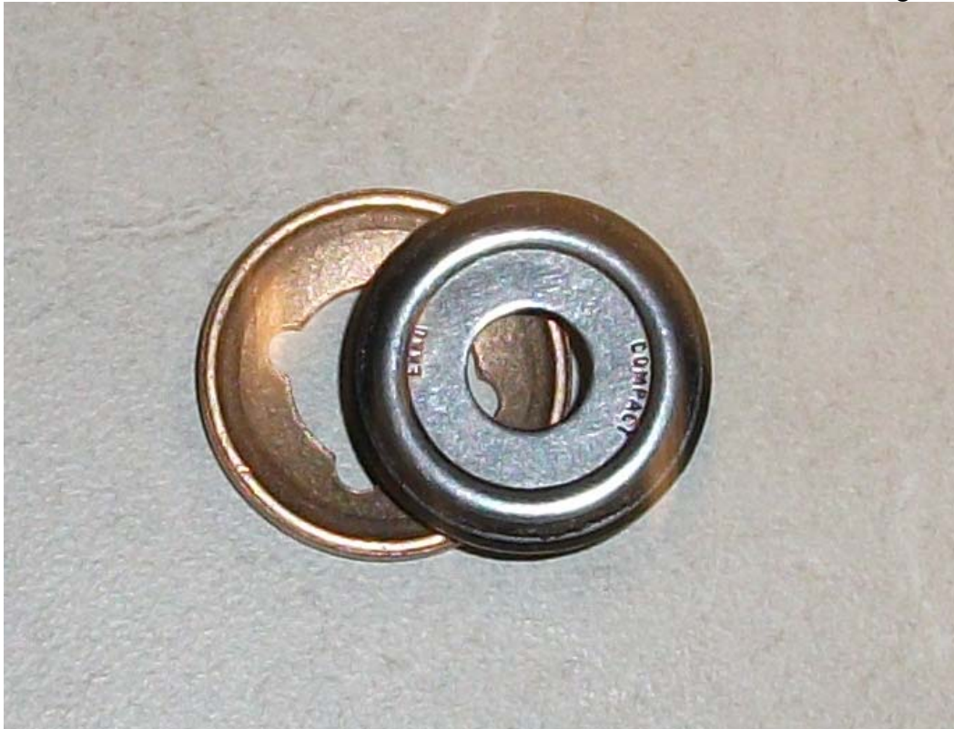
Figure 17: Ball bearings fitting into bushing
