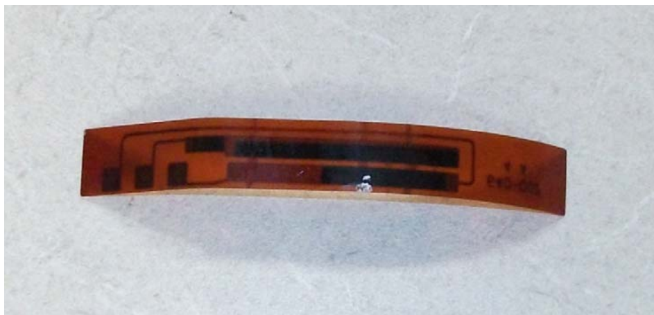
Figure 8: The back side of the strip shows the copper traces.
