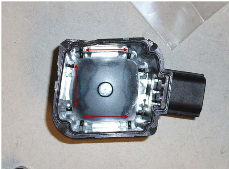
Figure 14: Arrows showing coil jumpers
